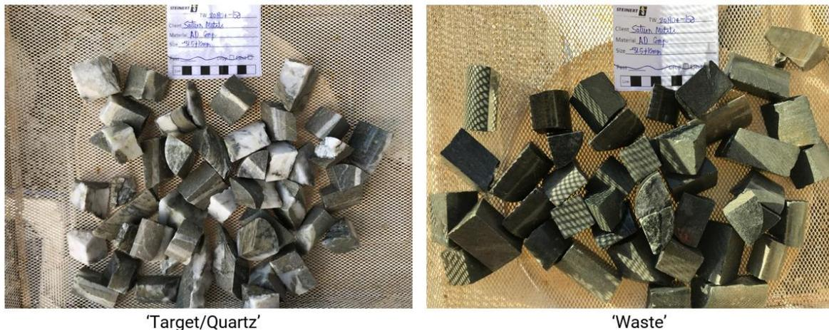
Figure 1. Hand sorted target quartz material used to set automatic optical 3D laser sorting parameters – sample id# AD
